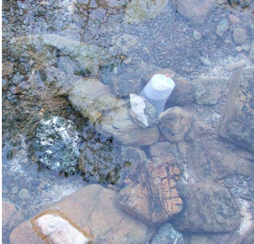
Figure 18: Hydrogen from reaction of serpentine with water collects in a bag (10 cm across) in a streambed in the Cedars area of California. Microbes living in the ground water have already reacted some of the hydrogen with \text{CO}_2 to make methane. Other microbes react the hydrogen with atmospheric oxygen near the surface. Photo by the author.
