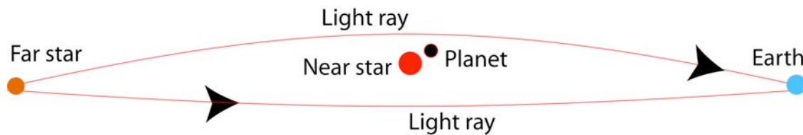
Figure 15: Schematic diagram of a nearer star acting as a gravitational lens for light from a distant star. The distant star appears to brighten when the alignment produces the lens. The presence of a planet produces additional focusing of light waves that pass near it. The amount of bending is grossly exaggerated in the diagram.
